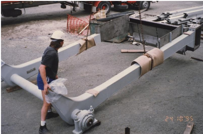
This sampler was designed for a 10,500 t/h conveyor
