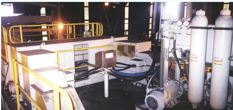
Hydraulic drive on large Swing Arm Sampler
