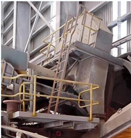
QHS Cross Belt Samplers are designed to collect representative samples of bulk materials from moving conveyor belts. These samplers comply with the requirements of Australian and International Standards for the sampling of bulk materials.
